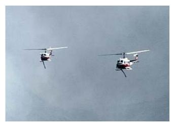
Initially, both helicopters were using their snorkels to refill with water while hovering. This is a difficult maneuver during windy conditions, as the pilot must hold the aircraft fairly stationary and level while refilling. To better support the helicopters, a ground fill operation was established. This enabled the helicopters to land and load water which is a much safer and effective procedure in wind conditions, as the pilots can land
