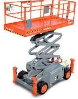
The age target for a scissor lift is 15 years, however, a review of actual service and repair costs will be used determine if replacement can be deferred.
