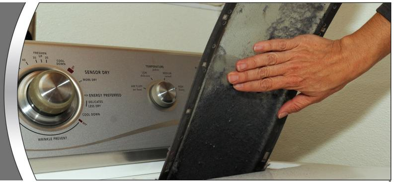
**The leading cause of home dryer fires is failure to clean them. Fires can occur if there is a build-up of lint in the dryer or the exhaust duct. Lint can block the flow of air which can cause excessive heat build-up, resulting in fire.**
