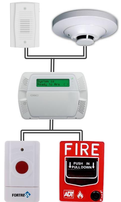
Combination fire & burglar alarm system with pull station or panic button activating smoke alarms and/or mini-horns
