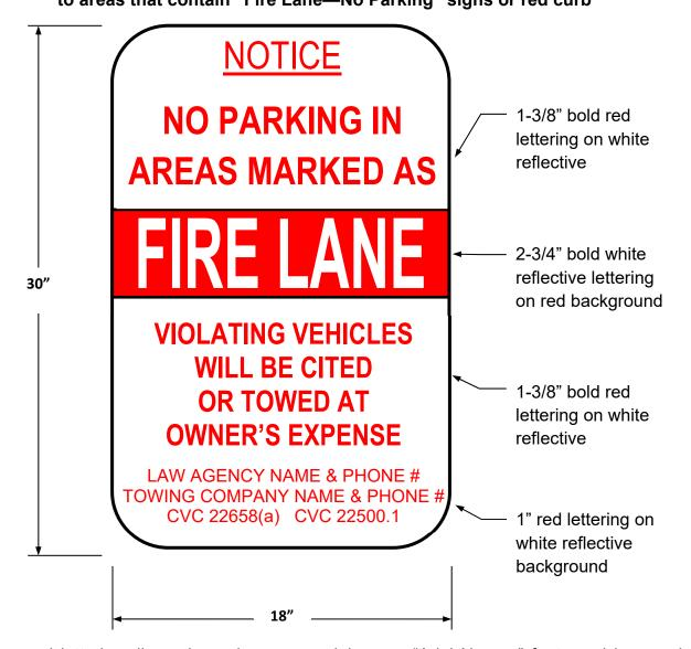
All sign and lettering dimensions shown are minimums. "Arial Narrow" font used in sample above, though other legible sans-serif fonts may be acceptable.
