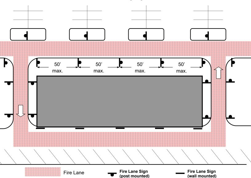
Signs are required within 3' of the end of each designated fire lane and spaced a maximum of 50' along the entire designated lane. One sign is required for each island adjacent to the fire lane.
