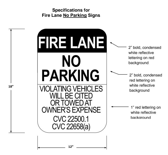
All sign and lettering dimensions shown are *minimums*. "Arial Narrow" font used in sample above, though other legible sans-serif fonts may be acceptable.
