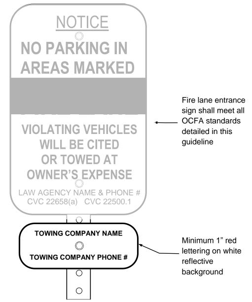
To facilitate periodic changes in towing company contracts, the towing company contact information may be posted on a separate sign mounted directly below the fire lane entrance sign instead of on the entrance sign itself. The method of attachment to the post shall not obscure the wording on either sign.
