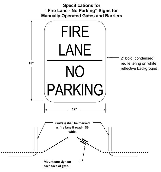
All sign and lettering dimensions shown are minimums. "Arial Narrow" font used in sample above, though other legible sans-serif fonts may be acceptable.
