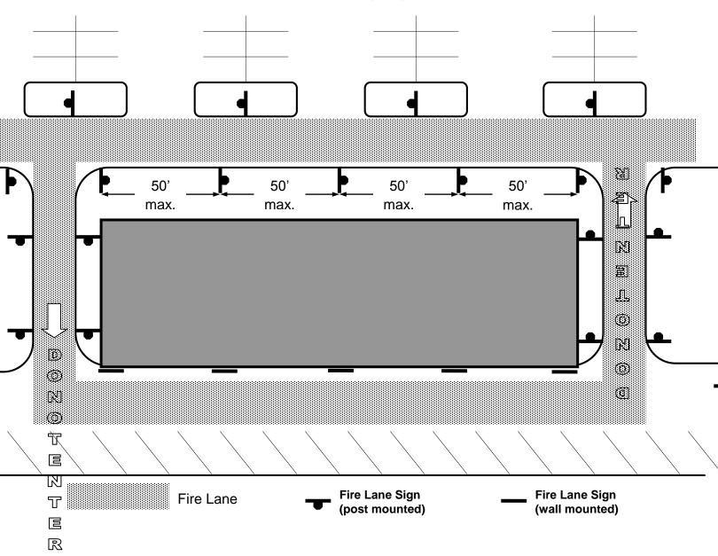
Signs are required within 3' of the end of each designated fire lane and spaced a maximum of 50' along the entire designated lane. One sign is required for each island adjacent to the fire lane.
