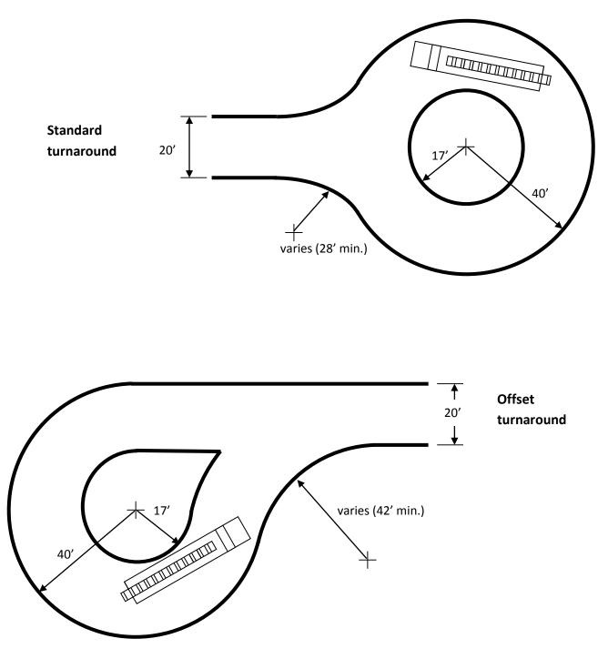
NOTE: Parking is not permitted in any of these hammerheads at the dimensions shown.
