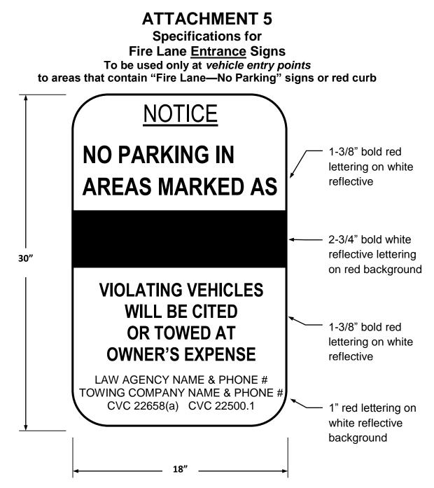
All sign and lettering dimensions shown are minimums. "Arial Narrow" font used in sample above, though other legible sans-serif fonts may be acceptable.
