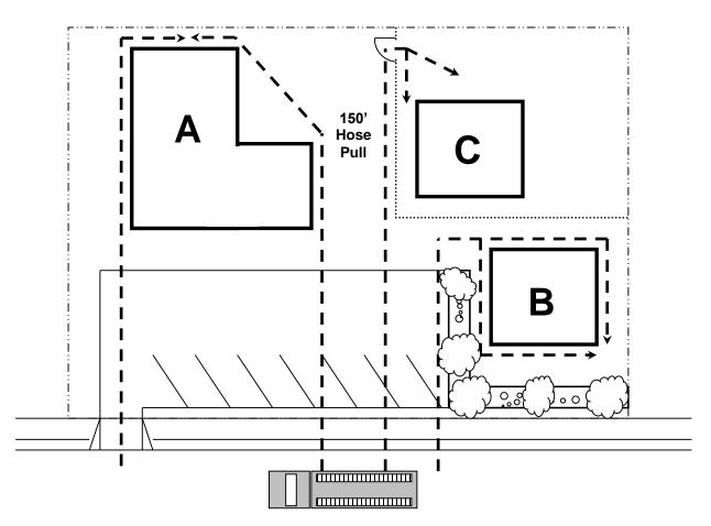
Assume that the parking lot is not accessible to fire apparatus due to turning radii and fire lane widths less than the required minimums.
